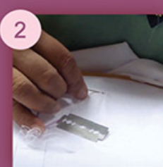
Remove thread with double-edged razor and needle
